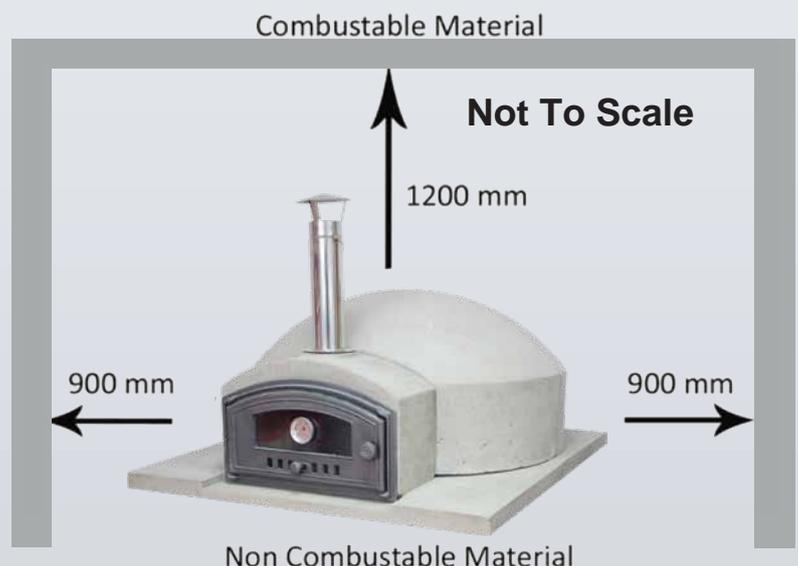
Example of required clearances for all ovens illustrated with a Pompeii model by way of example.
