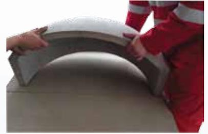
**3.** Place the back section 0 mm from the back of the base.
